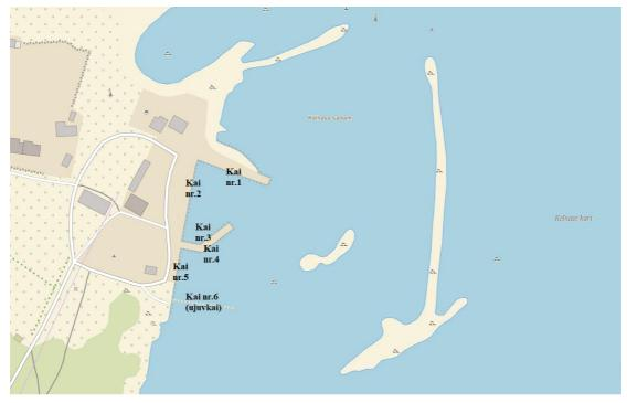
The conditions of the receipt of a ship are coordinated with the harbour master if the dimensions of the ship exceed the following: length 25.0 m; breadth 6.0 m, and draft 2.5 m. There is a respective territory to turn the ship around in the waters of the port with the diameter of 40 m and the depth of 3.1 m (EH2000).
